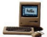
1984 Macintosh – the first PC with a graphic interface (instead of a command line interface)
